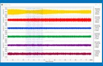
This plot shows history over a 6 month period. Each waveform contains about 150k samples and has been filtered to only display data from 0Hz to 1000Hz.
